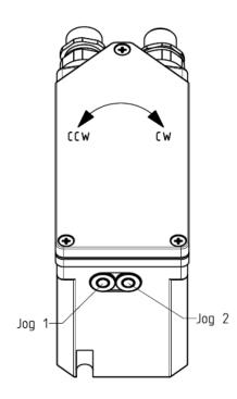
Holding both keys simultaneously for longer than 500 ms sets the actual drive position to 0.
